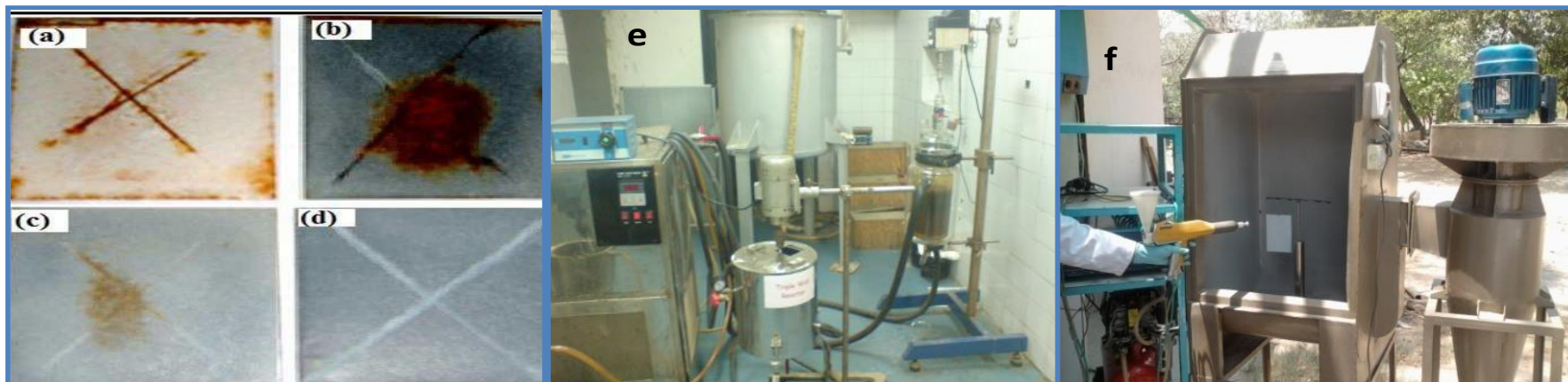
Figure 1: Salt spray images of powder coated sample (a) Epoxy coated, (b) PANI coated and 6% loading, (c) and (d) HPSC coated at 1.5 and 6% loading level, (e) pilot plant set up for the synthesis, (f) powder coating unit used for coating.
