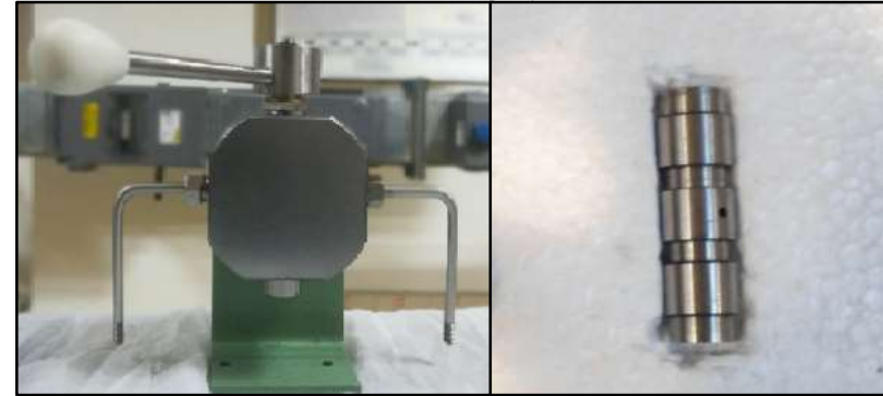
Fig: Snapshot of the developed Cross Floating Valve with its piston (Laboratory working model)
