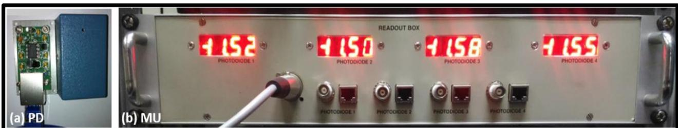
Figure 1: Photographs of the photodetector (PD) and monitor unit (MU). PD is assembled in a small metallic casing and the lid is kept open in this picture to show inside of it. MU has four channels and in this picture one of them is connected with the PD.
