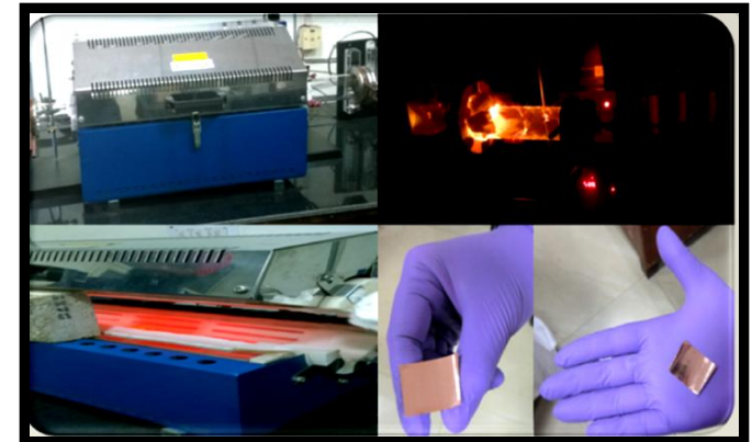
Figure: demonstrates the Graphene deposition on Cu substrate by CVD Set-up
