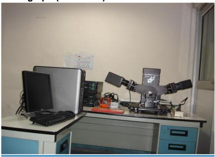
**Basic Principle:** The ellipsometer measures the change in polarization upon reflection or transmission. Since the polarization change depends upon the material properties i.e, thickness, dielectric function, refractive index, therefore fitting the ellipsometric data with the appropriate model results in extraction of the optical parameters of the thin film.
