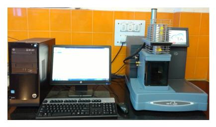
**Basic Principle:** TMA is based on the precise measurements of change in dimension as the sample is heated at a controlled rate.
