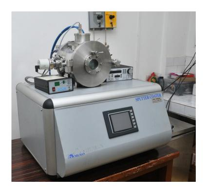
**Basic Principle :** In this process a gaseous plasma of typically inert gas ions such as Argon (Ar<sup>+</sup>) is created and the positive ions are accelerated by an electrical field to the target material which acts as the negatively charged electrode. The atoms from the target materials are ejected by bombardment of energetic ions and deposited on the desired substrate to form a film of the target materials.
