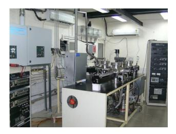
**Basic Principle :** PECVD is a process used to deposit thin films from a gas state to a solid state on a suitable substrate. Chemical reactions are involved in the process, which occur by creation of plasma of the reacting gases. The plasma is generally created by RF (AC) frequency discharge between two electrodes, the space between which is filled with the reacting gases.
