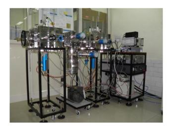
**Basic Principle :** In this process a gaseous plasma of typically inert gas ions such as Argon (Ar<sup>+</sup>) is created and the positive ions are accelerated by an electrical field to the target material which acts as the negatively charged electrode. The atoms from the target materials are ejected by bombardment of energetic ions and deposited on the desired substrate to form a film of the target materials.
