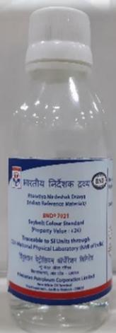
**Purpose:** Calibration of instruments, evaluation of test methods and performance verification of equipment used in the determination of Saybolt Colour.
