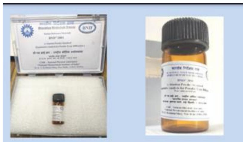
**PURPOSE:** BND<sup>®</sup> 2001, consists of an 'Alumina powder' (corundum structure), is an internal standard for intensity calibration of powder X-ray diffractometer (XRD).
