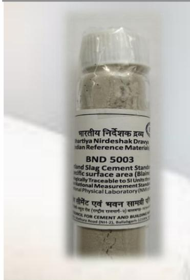
**Purpose:** BND<sup>®</sup> 5003, has been developed for calibrating Blaine Air Permeability Apparatus, developing in-house secondary reference materials for routine control and evaluating proficiency of analysts
