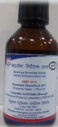
**Purpose:** Calibration of instruments and the evaluation of test methods used in the determination of Kinematic Viscosity.
