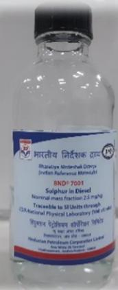
**Purpose:** Calibration of instruments and the evaluation of test methods used in the determination of total sulfur in gasoline or materials of similar matrix.
