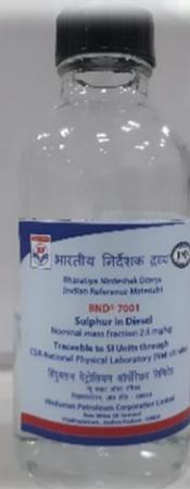
**Purpose:** Calibration of instruments and the evaluation of test methods used in the determination of total sulfur in kerosene or materials of similar matrix.
