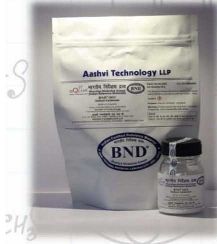
**Purpose:** Primary titrimetric standard for the standardization of volumetric standard solutions and validation of standard methods
