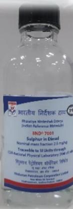
**Purpose:** Primary Standard for equipment performance check or calibration as per the standard test procedure.
