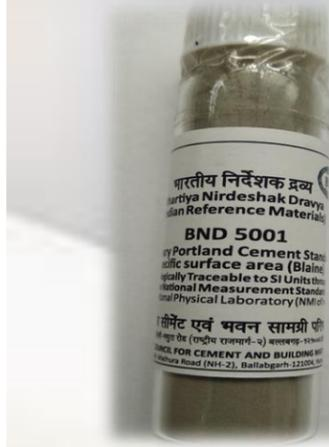
**Purpose:** BND<sup>®</sup> 5001, has been developed for calibrating Blaine Air Permeability Apparatus, developing in-house secondary reference materials for routine control and evaluating proficiency of analysts.
