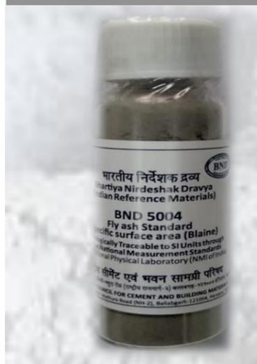
**Purpose:** BND<sup>®</sup> 5004, has been developed for calibrating Blaine Air Permeability Apparatus, developing in-house secondary reference materials for routine control and evaluating proficiency of analysts
