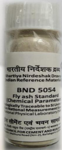
**Purpose:** BND<sup>®</sup> 5054, has been developed for evaluating proficiency of analysts, evaluating/comparing various test methods and calibration of equipment for analyzing alkalis for analysis of Fly ash.
