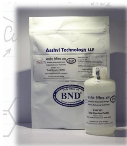
**Purpose:** Gravimetric standard for the validation of standard methods and calibration
