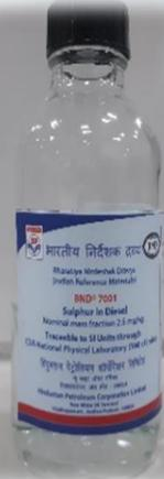
**Purpose:** Calibration of instruments and the evaluation of test methods used in the determination of total sulfur in Gasoline or materials of similar matrix.
