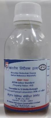
**Purpose:** Calibration of instruments and the evaluation of test methods used in the determination of total acid number in Mineral oil / Mineral oil matrix matching material.
