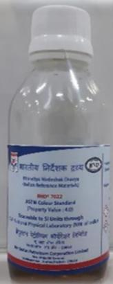
**Purpose:** Calibration of instruments and the evaluation of test methods used in the determination of total base number in Mineral oil / Mineral oil matrix matching material.
