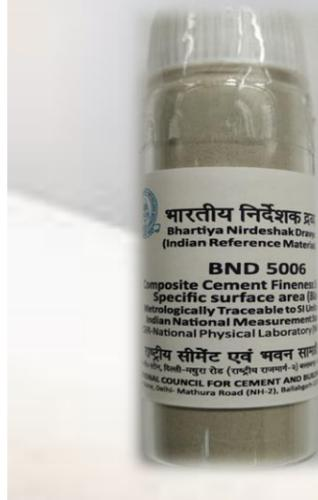
**Purpose:** BND<sup>®</sup> 5006, has been developed for calibrating Blaine Air Permeability Apparatus, developing in-house secondary reference materials for routine control and evaluating proficiency of analysts.
