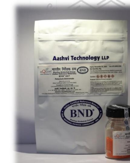
**Purpose:** Primary titrimetric standard for the standardization of volumetric standard solutions and validation of standard methods.
