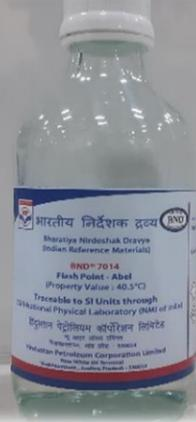
**Purpose:** Calibration of instruments and the evaluation of test methods used in the determination of Flash Point (Abel).
