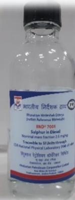
**Purpose:** Calibration of instruments and the evaluation of test methods used in the determination of total sulfur in Gasoline or materials of similar matrix.
