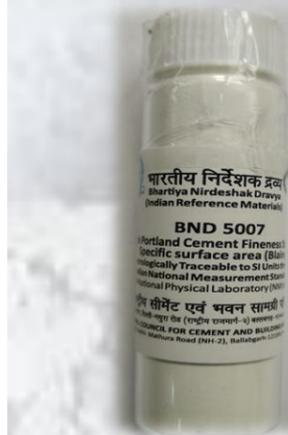
**Purpose:** BND<sup>®</sup> 5007, has been developed for calibrating Blaine Air Permeability Apparatus, developing in-house secondary reference materials for routine control and evaluating proficiency of analysts.
