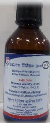
**Purpose:** Calibration of instruments and the evaluation of test methods used in the determination of Kinematic Viscosity.
