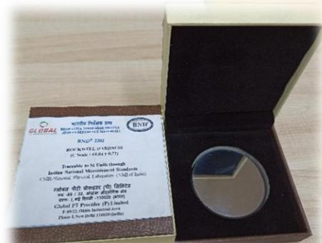
**Purpose:** Rockwell Hardness reference blocks are used for periodic check or verification of hardness testing machines.
