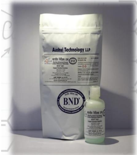
**Purpose:** Primary calibration standard for the quantitative determination of copper, calibration of instruments and validation of method for the quantification/ characterization of measurand.
