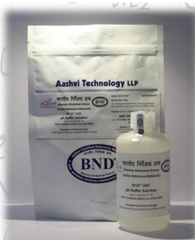
**Purpose:** Calibration standard for calibration of pH instruments and validation of method for determination of the pH value.
