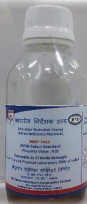
**Purpose:** Use for the evaluation of test methods, performance verification of equipment used in the determination of Colour ASTM
