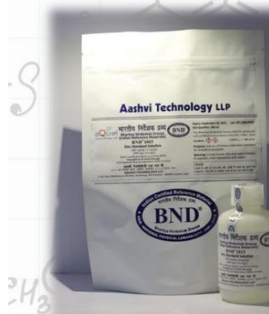
**Purpose:** Primary Calibration standard for quantitative determination of Zinc calibration of instrument and validation of method for the quantification/ characterization of the measurand.
