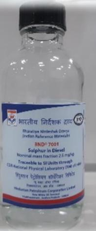
**Purpose:** Calibration of instruments and the evaluation of test methods used in the determination of total sulfur in gasoline or materials of similar matrix.
