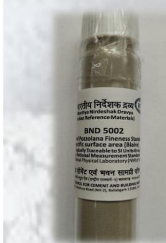
**Purpose:** BND<sup>®</sup> 5002, has been developed for calibrating Blaine Air Permeability Apparatus, developing in-house secondary reference materials for routine control and evaluating proficiency of analysts.
