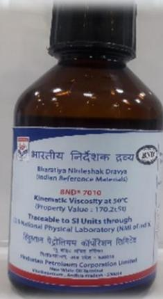
**Purpose:** Calibration of instruments and the evaluation of test methods used in the determination of Kinematic Viscosity.
