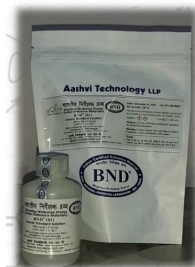
**Purpose:** Primary Calibration standard for quantitative determination of Arsenic calibration of instrument and validation of method for the quantification/ characterization of the measurand.
