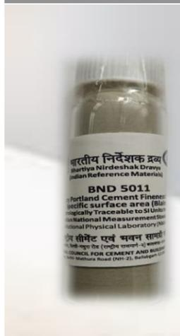
**Purpose:** BND<sup>®</sup> 5011, has been developed for calibrating Blaine Air Permeability Apparatus, developing in-house secondary reference materials for routine control and evaluating proficiency of analysts.
