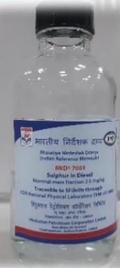
**Purpose:** Calibration of instruments and the evaluation of test methods used in the determination of total sulfur in Gasoline or materials of similar matrix.
