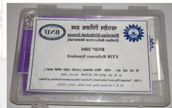
**PURPOSE:** BND<sup>®</sup> 2004 is meant for the calibration of Fourier Transform Infrared (FTIR) Spectrometer which is being routinely used in chemical and pharmaceutical industry.
