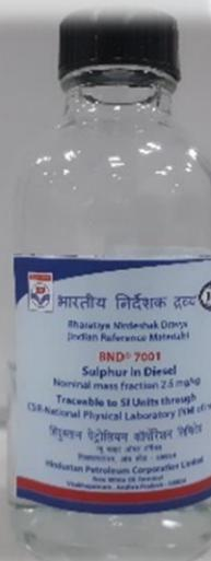
**Purpose:** Calibration of instruments and the evaluation of test methods used in the determination of total sulfur in diesel or materials of similar matrix.
