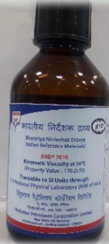
**Purpose:** Calibration of instruments and the evaluation of test methods used in the determination of Kinematic Viscosity.
