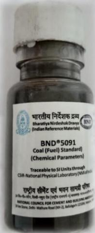
**Purpose:** BND<sup>®</sup> 5091, is intended to use as a primary standard for calibration of instruments and validation of method for the characterization of the measurand for the analysis of coal.
