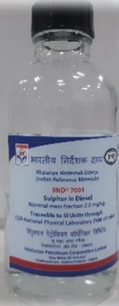
**Purpose:** Calibration of instruments and the evaluation of test methods used in the determination of total sulfur in diesel or materials of similar matrix.
