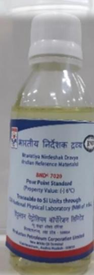
**Purpose:** Use for the evaluation of test methods Pour Point of Petroleum Oils or oils of similar matrix
