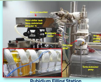
Rubidium Bulbs containing Natural Rubidium: Mixture of Rb-87 (27.8%) and Rb-85 (72.2%), Buffer gas: 2 \pm 0.1 Torr Krypton gas of 99.999% purity.
