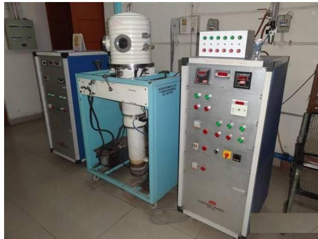
**Basic Principle:** In thermal Evaporation technique basically, material is heated in a vacuum chamber until its surface atoms have sufficient energy to leave the surface. At this point they will traverse the vacuum chamber, and coat a substrate positioned above the evaporating material.
