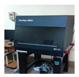
**Basic Principle:** A contact profilometer uses a diamond stylus, which is moved vertically and laterally in contact with the sample for a specified distance. It precisely measures small variations in stylus displacement as a function of position. This technique is a real direct measurement of surface height or thickness of the sample.
