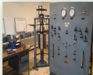
NPL-H1: Primary Pressure Standard for 1GPa
