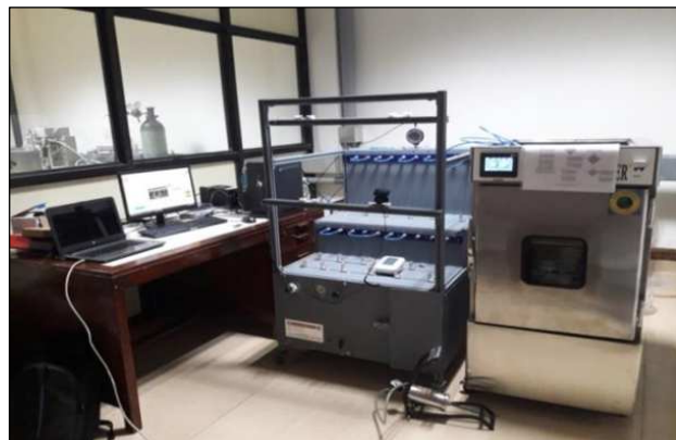
Calibration/testing system for the non-invasive blood pressure monitoring system CSIR-NPL
