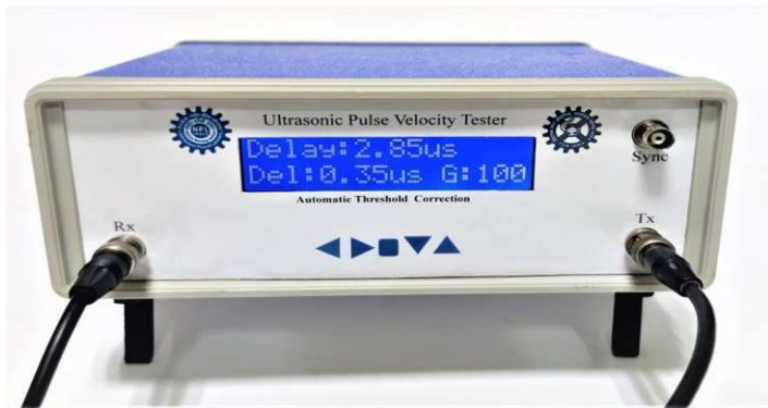
Ultrasonic pulse velocity tester developed at CSIR-NPL
