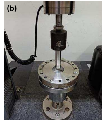
(a) Components of ball burst test set-up (b) Indigenously developed Ball burst test set-up for bursting strength measurement of surgical gowns platelets
