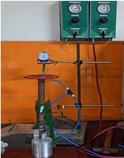
Hydrostatic resistance test set-up as per ASTM D-751
