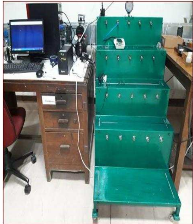
A Mechanical Blood Pressure Measuring System for Legal Metrology Department, Govt. of India (Some of the fabrication and fitting works were carried out at Central Workshop)
