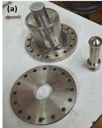
(a) Components of ball burst test set-up (b) Indigenously developed Ball burst test set-up for bursting strength measurement of surgical gowns platelets
