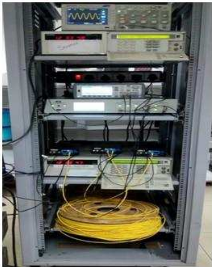
In house experimental setup of the White Rabbit network based optical fibre link and time delay variation between the two ends of the optical fibre link
