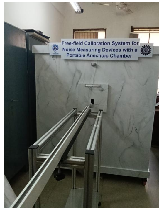
Fig.1: (a) Schematic of Free-field calibration facility (Left); Pictorial view of Developed Free-field calibration facility at CSIR-NPL (Right)
